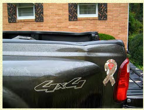
Jumping out of the truck we discovered that the fifth wheel had slipped off the hitch and landed on the sides of the truck. ):
